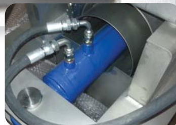
Piston with sleeve and slotted dewatering zone
